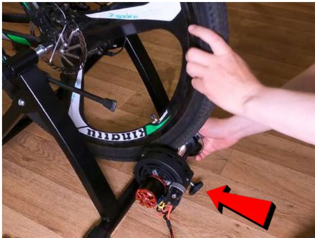
15. Test that the wheel doesn't slip on the roller. If it does - increase the traction - but not too tight!
