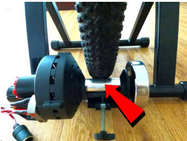
9. Make sure the tyre is in the middle of the roller
