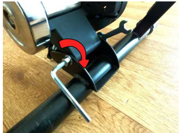
4. Use the tools to attach the generator - but not too tight!
