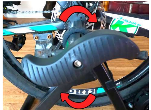
10. Turn both the handles to clamp the rear wheel in place
