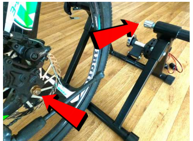
8. Line up the bolt on the back wheel with the sockets
