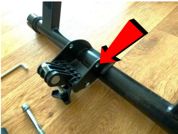
3. The large bolt goes through here to attach the generator
