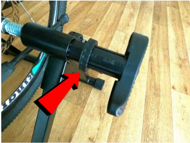
13. The wheel is now locked safely in place
